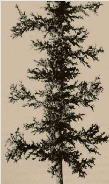
Laboratory core flow test results showing branching wormhole created in a limestone core using SXE acid.
